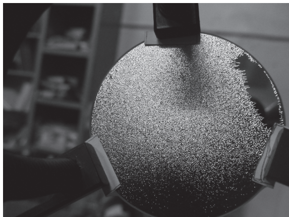
Figure 3. Exfoliation of the MM structure (the first layer on a quartz substrate is antimony).
