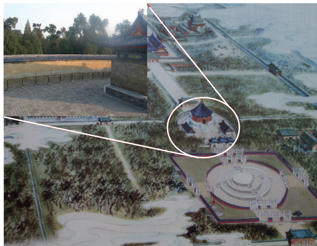
Figure 4. Echo Wall in the Temple of Heaven, Beijing, as an example of an acoustic WGM resonator: plan image and photograph (inset).
