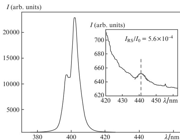
**Figure 7.** Lidar signal spectrum in the range of altitudes of 75–2000 m. In the inset shown is the spectrum region corresponding to the Raman line of nitrogen (the location of its maximum is indicated by the dashed vertical line).
