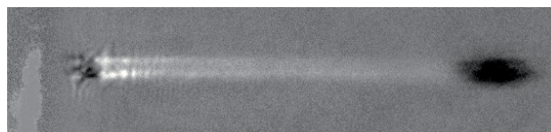
Figure 2. Interference image illustrating the propagation of a femtosecond pulse (from left to right) in diamond (266 nm, 120 fs, 90 nJ). One can see the surface of the sample (at left), the wave packet proper (black) and the plasma channel (white). The horizontal size of the image is 300 \mu\text{m} .
