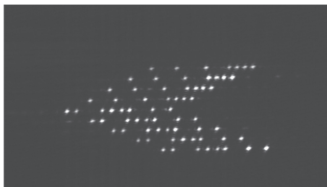
Figure 10. Image of the test object in the form of the input data page fragment, reconstructed from a single one-dimensional Fourier subhologram.
