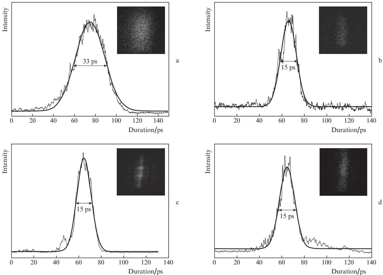
**Figure 2.** Pulses of radiation recorded with the streak camera for the master oscillator (a); at the input of the amplifier (193 nm) (b), at the amplifier output (193 nm) in the single-pass (c) and three-pass scheme (d).
