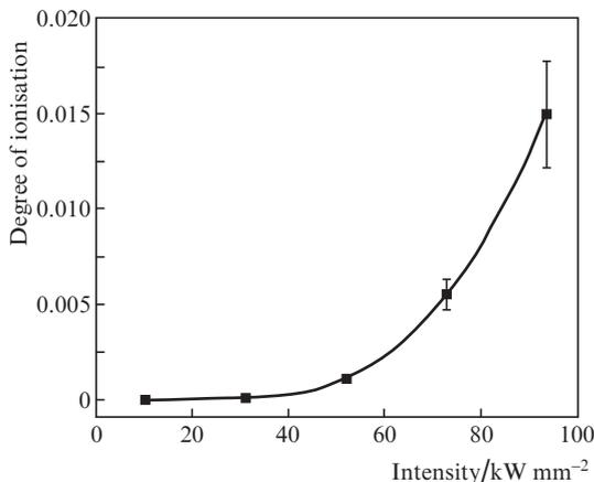
**Figure 7.** Degree of ionisation of the vapour-plasma plume as a function of the laser radiation intensity.
