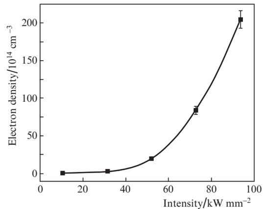
**Figure 8.** Free-electron density in the welding plume plasma as a function of the laser radiation intensity.
