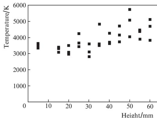
**Figure 10.** Height dependence of the welding plume temperature in the welding of titanium.
