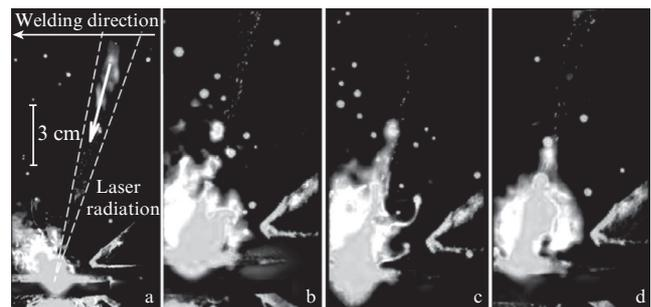
**Figure 3.** Frames of high-speed video filming of the welding plume when laser radiation was incident on the metal surface at an angle of 15°.
