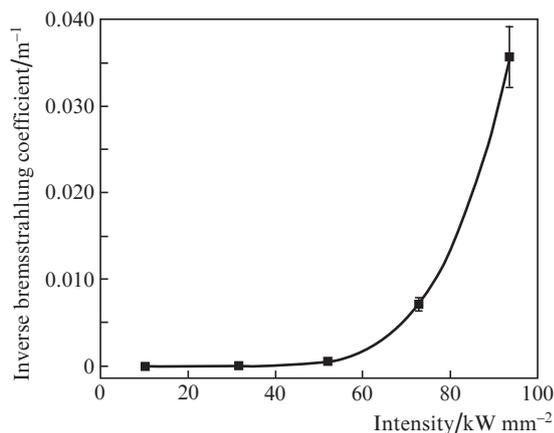
**Figure 9.** Dependence of the inverse bremsstrahlung coefficient for the vapour-plasma plume on the laser radiation intensity.
