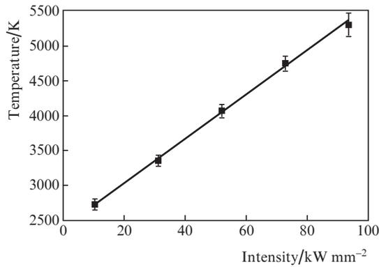
**Figure 6.** Dependence of the vapour-plasma plume temperature on the intensity of laser radiation.
