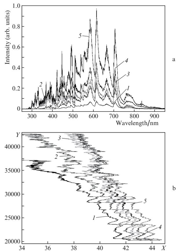
**Figure 5.** Emission spectra of the vapour-plasma plume measured for laser radiation intensities of (1) 10, (2) 31, (3) 52, (4) 73 and (5) 94 kW mm<sup>-2</sup> (a) and represented in the new coordinates (b).
