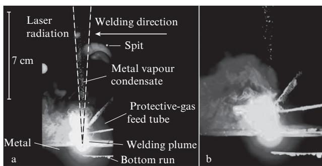
**Figure 2.** Frame of high-speed video filming of the welding plume for normal incidence of radiation on the metal (a) and magnified image of the welding plume (b).
