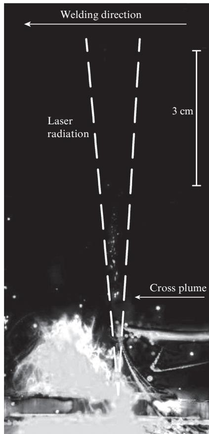
**Figure 4.** Frame of high-speed video filming of titanium welding using the blow-off of the welding plume with a cross plume of compressed air.
