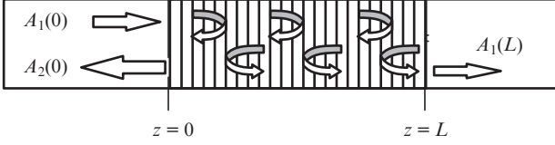
Figure 1. Schematic diagram of wave propagation in an active one-dimensional PC.
