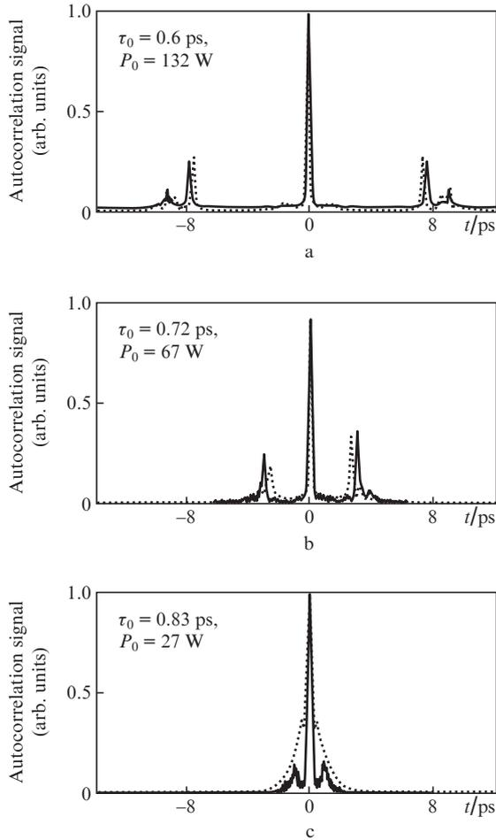
**Figure 5.** Measured (solid lines) and calculated (dotted lines) autocorrelation traces obtained at the DSF output at different parameters of the pulse launched into the fibre.
