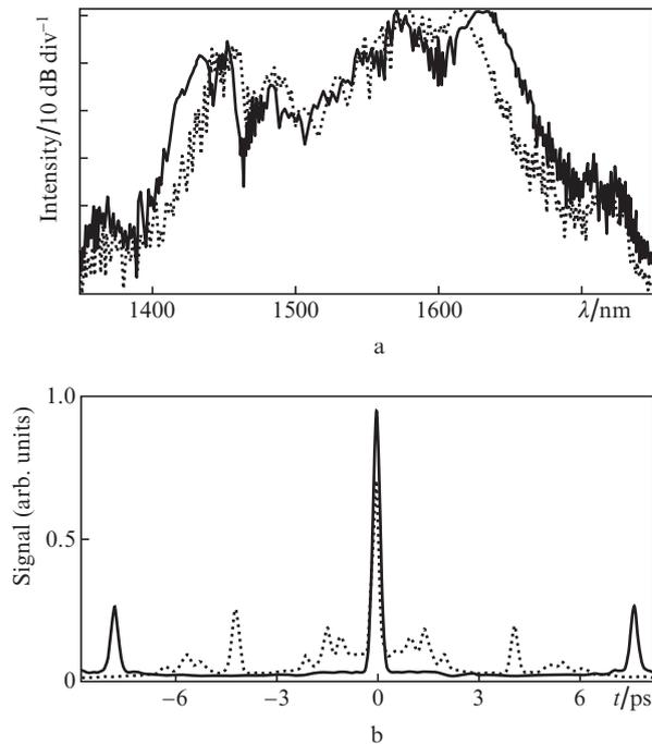
**Figure 3.** (a) Emission spectra and (b) autocorrelation traces at the output of the inhomogeneous DSF. The solid lines represent a forward pass (decreasing fibre diameter) and the dotted lines represent a backward pass.
