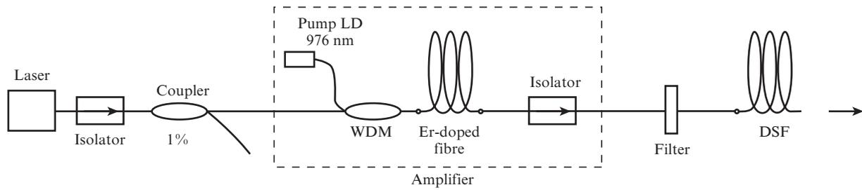
**Figure 1.** Schematic of the experimental setup.
