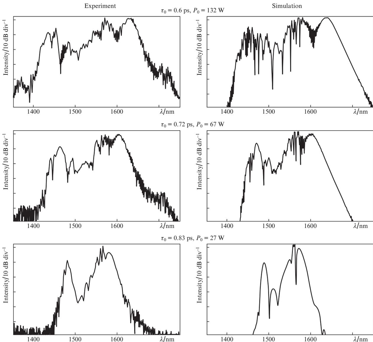
**Figure 4.** Measured (left) and calculated (right) spectra obtained at the DSF output at different input pulse parameters.
