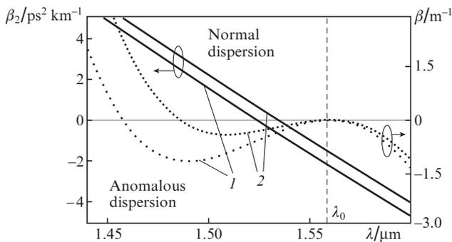
**Figure 2.** GVD curves of the DSF under study (solid lines) and  $\beta = \frac{1}{2}\beta_2(\omega_0)(\omega - \omega_0)^2 + \frac{1}{6}\beta_3(\omega_0)(\omega - \omega_0)^3$  dispersion curves relative to the pulse carrier frequency  $\omega_0$  corresponding to  $\lambda_0 = 1.56 \mu\text{m}$  (dotted lines) at fibre diameters of (1) 86.9 and (2) 86.1  $\mu\text{m}$ .
