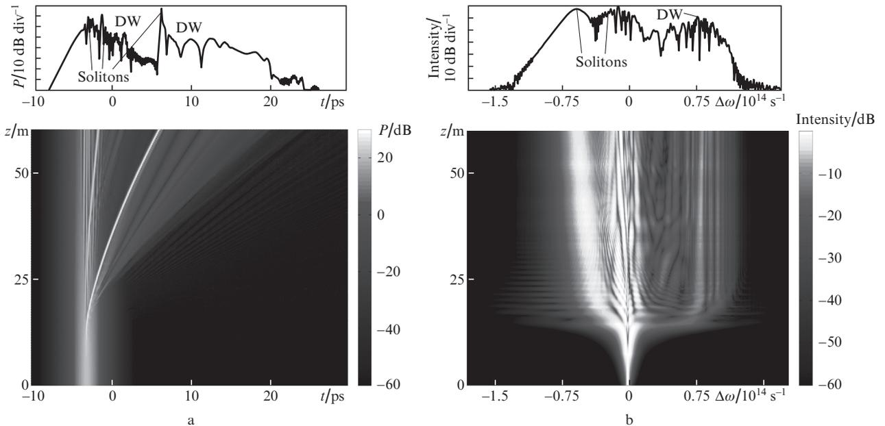
**Figure 6.** Numerical simulation results: evolution of the (a) temporal envelope and (b) spectrum of a primary pulse ( $\tau_0 = 0.6$  ps,  $P_0 = 132$  W) propagating through the fibre; DW = dispersive wave.
