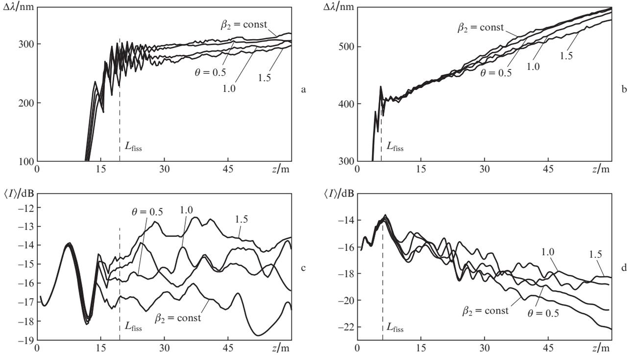
**Figure 9.** Numerical simulation results: (a, b) 30-dB bandwidth as a function of longitudinal coordinate for the supercontinuum generated in a fibre with decreasing GVD,  $\beta_2 = \beta_{20}(1 - \theta z/L)$  ( $L = 60$  m); (c, d) average logarithm of the intensity within the band in question. Primary-pulse parameters: (a, b)  $\tau_0 = 0.6$  ps,  $P_0 = 132$  W; (c, d)  $\tau_0 = 0.3$  ps,  $P_0 = 528$  W.
