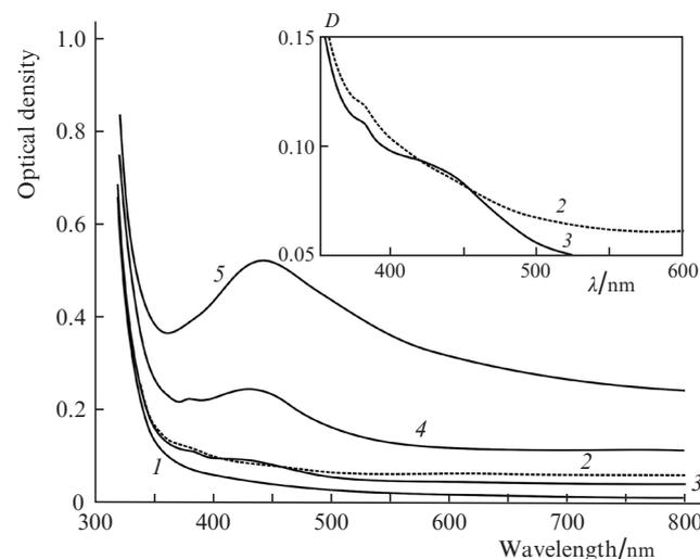
**Figure 2.** Spectra of the integral optical density  $D$  of the glass before (1) and after the irradiation with the CO<sub>2</sub> laser with  $E =$  (2) 0.6, (3) 0.95, (4) 3.8 and (5) 8.5  $\text{J cm}^{-2}$ . The inset shows curves (2) and (3) in the magnified scale.
