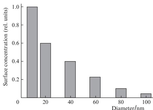
**Figure 4.** Normalised size distribution of silver nanoparticles at the outer side of the ring.
