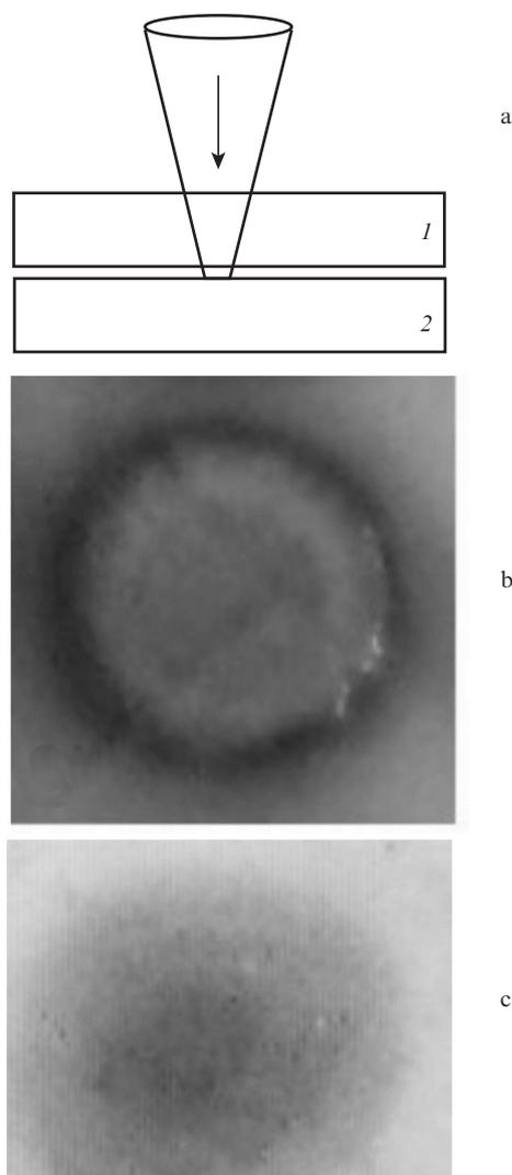
**Figure 5.** (a) Schematic diagram of irradiation of the glass with the CO<sub>2</sub> laser [(1) KBr or ZnSe plate, (2) glass doped with silver ions] and a photograph of the laser torch trace on the plates of (b) KBr and (c) ZnSe. The photographs were obtained in reflected light;  $E = 3.8 \text{ J cm}^{-2}$ .
