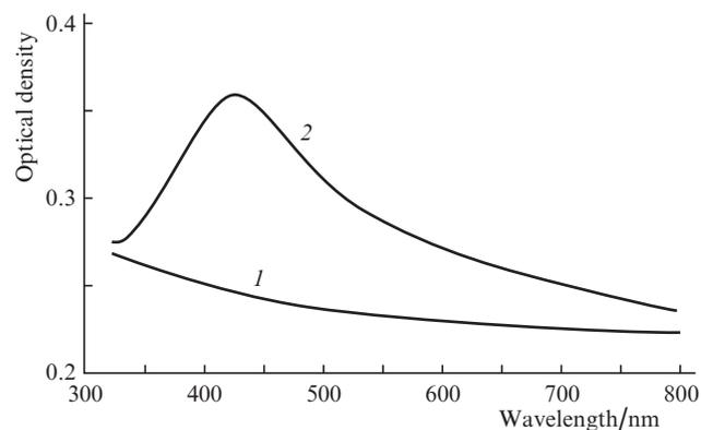
**Figure 6.** Spectra of integral optical density of KBr plate (1) before and (2) after irradiation of the glass doped with silver ions with a CO<sub>2</sub> laser;  $E = 3.8 \text{ J cm}^{-2}$ .
