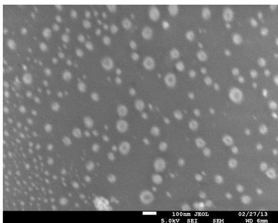
**Figure 3.** SEM image of silver nanoparticles at the outer side of the ring at  $E = 3.8 \text{ J cm}^{-2}$ .
