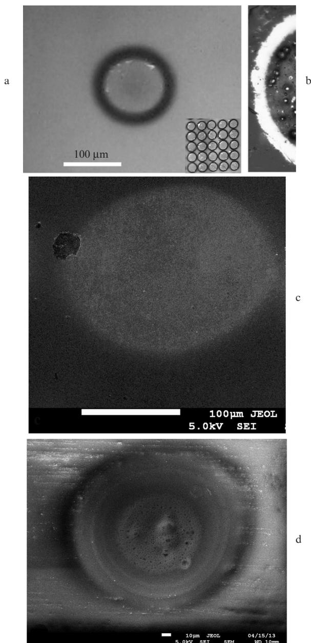
**Figure 1.** Photographs of (a) the irradiated glass zone at  $E = 0.95\text{ J cm}^{-2}$  (the inset shows a fragment of the matrix used for measuring the integral optical density) and (b) the edge of the irradiated glass zone at  $E = 8.5\text{ J cm}^{-2}$ , as well as SEM images of (c) the irradiated zone at  $E = 0.95\text{ J cm}^{-2}$  and (d) a crater at  $E = 3.8\text{ J cm}^{-2}$ . The photographs in Figs 1a and 1b are obtained in reflected light using an optical microscope.
