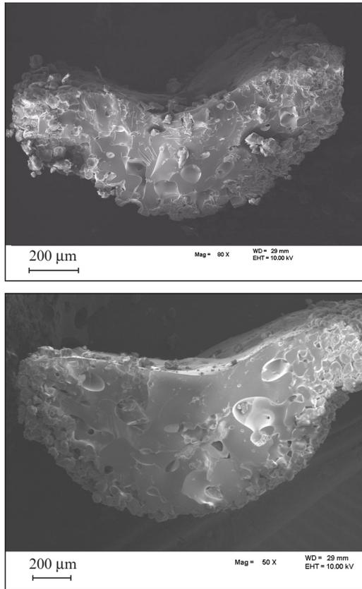
**Figure 6.** Microphotographs of cross sections of polymer filaments sintered at  $W =$  (a) 0.3 and (b) 1.0 W in a polymer powder wetted with water.
