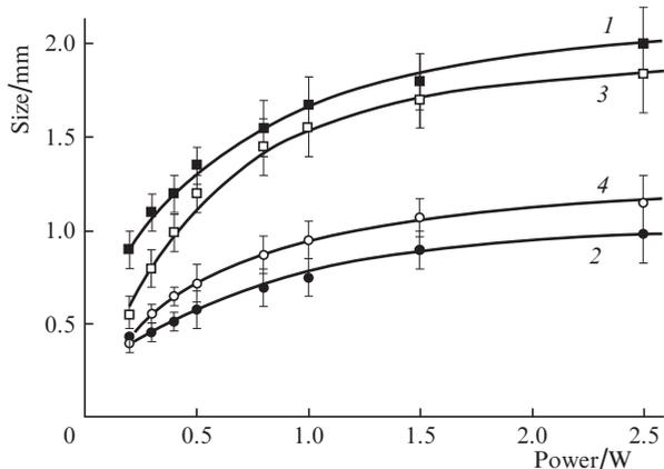
**Figure 10.** Dependence of the cross section width of sintered structures (1, 3) and the sintering depth (2, 4) on the laser radiation power for the sintering in water-wetted polymer powder (1, 2) and in air (3, 4).
