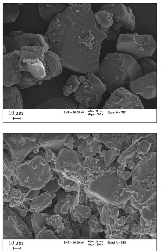
**Figure 2.** Microphotographs of the source powder of (a) the polymer and (b) the powder treated with the HA solution.
