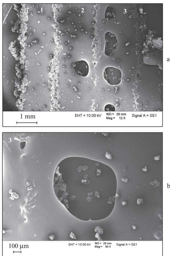
**Figure 9.** Microphotographs of (a) the structures sintered at a laser beam scanning velocity  $1 \text{ mm s}^{-1}$  and a radiation power ( $I$ ) 0.5, (2) 1.0 and (3) 1.5 W (3), and (b) the magnified fragment of the structure sintered at  $W = 1.5 \text{ W}$ .
