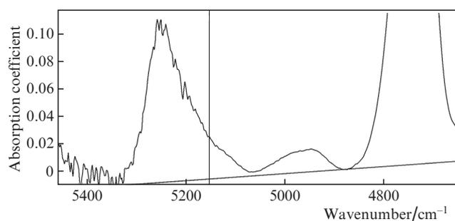
**Figure 1.** IR absorption spectrum of the PDLG 7502 film. The position of the wavenumber  $5155 \text{ cm}^{-1}$ , corresponding to  $\lambda = 1.94 \mu\text{m}$ , is shown by a vertical line. The sloped straight line is the baseline.
