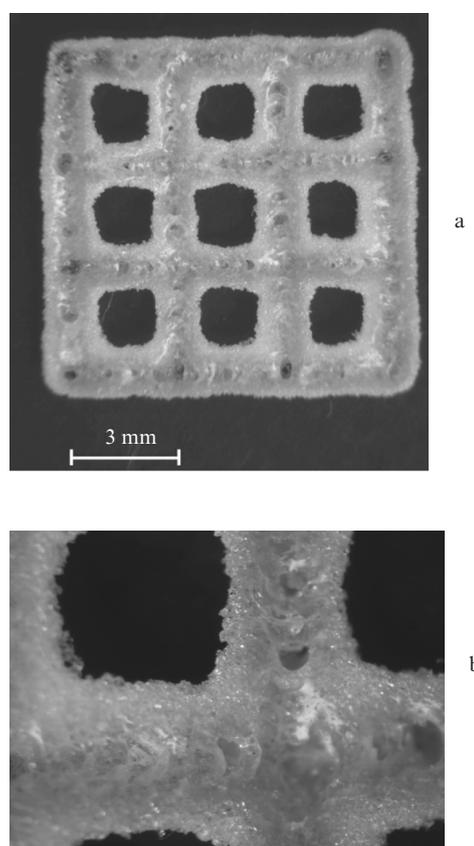
**Figure 11.** (a) Photograph of the matrix structure sintered in the wetted powder at  $W = 0.8 \text{ W}$  and (b) its magnified fragment.
