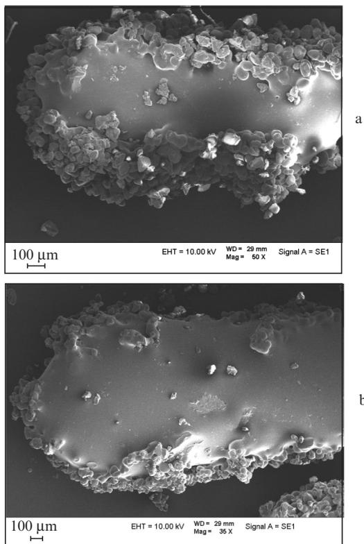
**Figure 7.** Microphotographs of the fragments of polymer filaments sintered in dry powder at  $W =$  (a) 0.4 and (b) 0.8 W.
