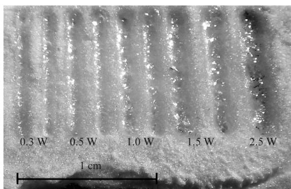
**Figure 4.** Photograph of polymer filaments sintered in a water-wetted powder at different laser radiation powers. The powder layer thickness is 1 mm.
