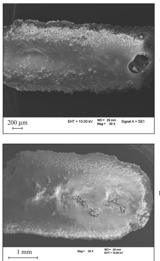
**Figure 5.** Microphotographs of the fragments of polymer filaments sintered in a polymer powder wetted with water at  $W =$  (a) 0.3 and (b) 2.5 W.
