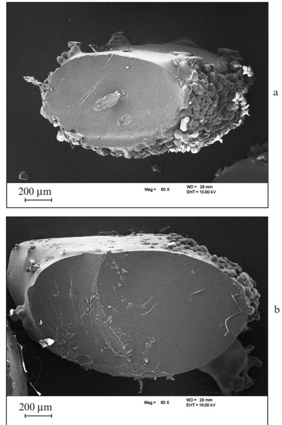
**Figure 8.** Microphotographs of cross sections of polymer filaments sintered in dry powder at  $W =$  (a) 0.4 and (b) 0.8 W.
