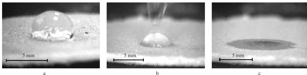
**Figure 3.** Photographs of water drops (a) on the surface of the intact polymer powder and (b–c) on the powder surface after the treatment of its particles with the HA solution: (b) the moment of drop application and (c) the drop after 10 s.
