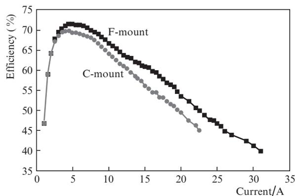
**Figure 2.** Total efficiency calculated using (1) as a function of pump current for laser diodes (980 nm, 95  $\mu\text{m}$ , 4 mm) on copper C- and F-mounts.
