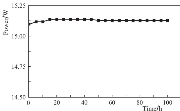
**Figure 3.** Short-term (100 h) reliable-operation test of a laser diode on an F-mount at an output power of 15 W.
