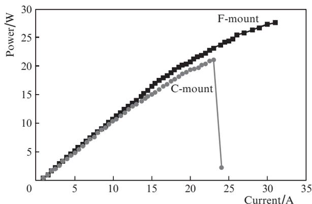
**Figure 1.** Light–current curves of laser diodes (wavelength, 980 nm; stripe contact width, 95  $\mu\text{m}$ ; cavity length, 4 mm) on copper C- and F-mounts.
