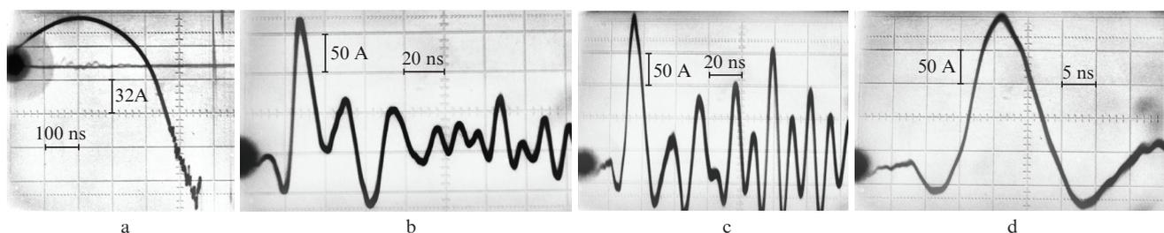
**Figure 2.** Oscillograms of current pulses in the chain of diodes (6) (a) and the AE at  $C_t = 120$  (b) and  $70 \text{ pF}$  (c, d).
