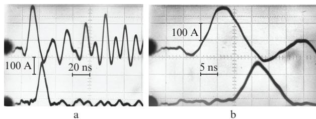
Figure 3. Oscillograms of current pulses (upper curve) and lasing pulses (lower curve).
