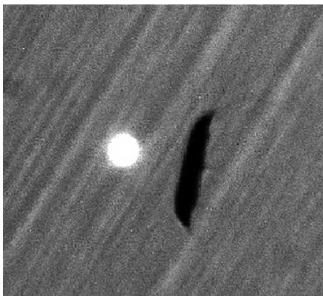
Figure 5. Shadow image of the deformed droplet with the diameter 60 μm (the frame size 600 × 550 μm); λ = 532 nm, the pulse energy 20 mJ, Δτ = 25 ns.
