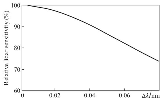
**Figure 4.** Relative sensitivity of the methane detecting lidar as a function of the line width of the lidar radiation  $\Delta\lambda$ .
