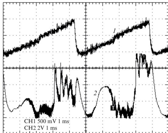
**Figure 2.** Signals from photodetectors 1 (1) and 2 (2). Signal (2) is produced by reflection of light from a grey brick placed at a distance of 100 m from the lidar. The output power of the lidar is 2.5 W.
