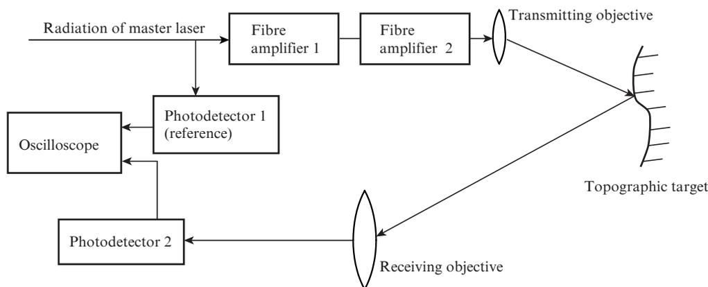
Figure 1. Block diagram of the setup for methane detection.
