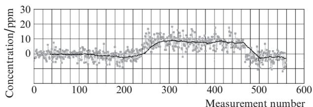
**Figure 5.** Measured methane concentrations in the calibrated cuvette (points) and their approximation (solid curve). The distance to the target is 1.2 km.
