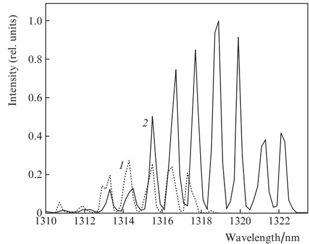
**Figure 2.** Disk laser spectra at pump powers of (1) 14.1 and (2) 21.2 W.
