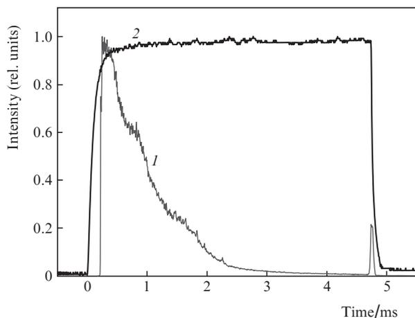
**Figure 4.** Laser pulse at a wavelength of 1314.3 nm (1) and pump pulse (2).
