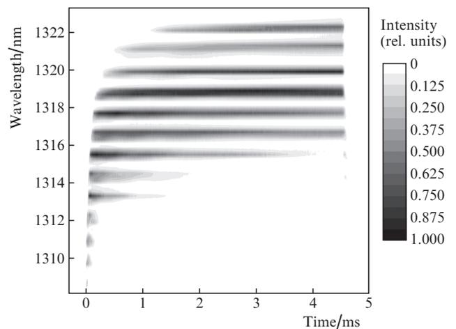
**Figure 3.** Time dependences of the laser spectrum upon pulsed pumping.
