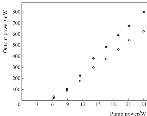
**Figure 6.** Dependences of the second harmonic ( $\lambda = 660$  nm) power of the SDL on the pump power in the pulsed (●) and cw (○) regimes.
