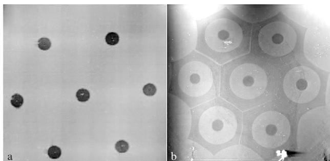
**Figure 3.** Atomic force microscopy images of the end faces of the fibres (a) without and (b) with a reduced-index layer.
