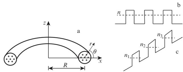
**Figure 2.** (a) Multicore fibre bent to a radius  $R$  and refractive index profiles of (b) a straight and (c) a bent fibre.
