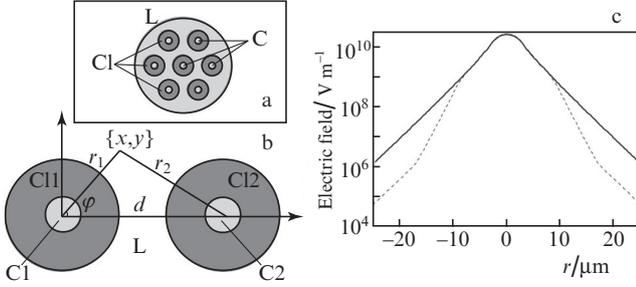
**Figure 1.** (a) Cross section of a multicore fibre, (b) waveguiding system under consideration and (c) mode field distributions across the fibres with (dashed line) and without (solid line) a reduced-index layer.
