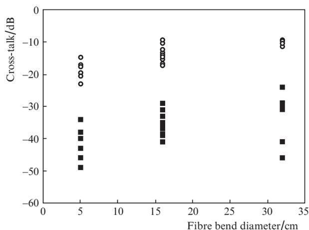
**Figure 4.** Cross-talk between the central and peripheral cores as a function of fibre bend diameter for the fibres with (■) and without (○) a reduced-index layer.
