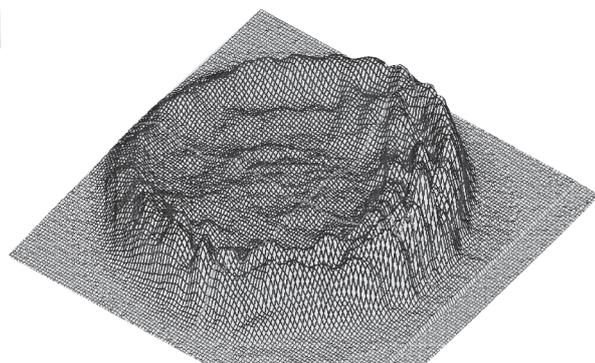
**Figure 4.** Profile of the output beam of the inductive HF laser. The charge voltage is  $U_{\text{ch}} = 25$  kV, the mixture is  $\text{He}:\text{H}_2:\text{NF}_3 = 45:1:4$ .
