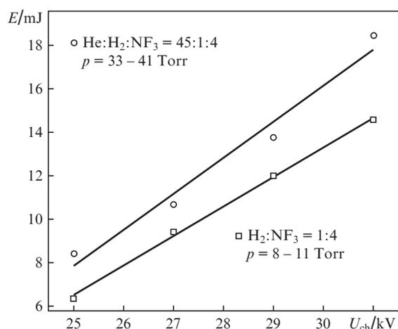
**Figure 1.** Output energy  $E$  vs. the charge voltage  $U_{ch}$  of the inductive HF laser with two- and three-component mixtures.
