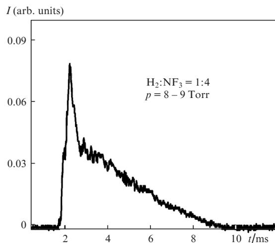
**Figure 2.** Oscillogram of an output pulse of the HF laser. The charge voltage is  $U_{ch} = 25$  kV.
