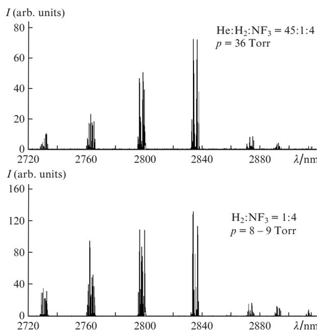
**Figure 3.** Emission spectrum of the inductive HF laser. The charge voltage is  $U_{ch} = 25$  kV.
