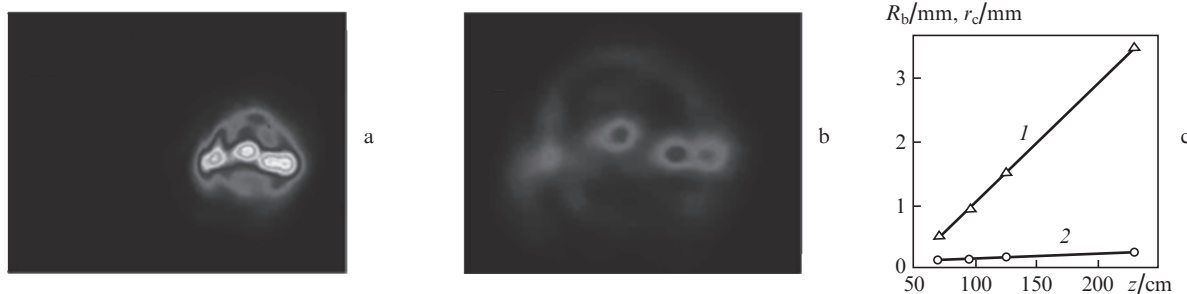
Figure 2. Transverse profile distributions of the radiation energy density with E_0 = 3.9 mJ at the distances from the linear beam focus z = (a) 125 and (b) 230 cm at f = 52 cm; (c) dependence of the effective radius of (1) the entire beam R_b and (2) PFC r_c on the distance z from the linear focus.
