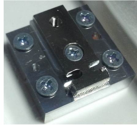
Figure 3. Photograph of quasi-cw LDA5 on a C–S mount emitting at 808-nm with a power of 300 W.
