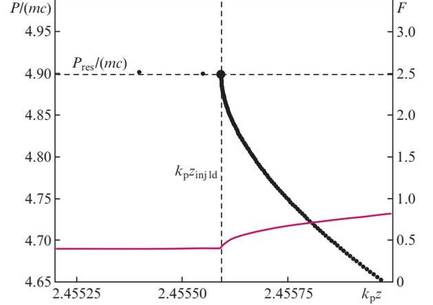
**Figure 1.** Electron distribution on the phase plane  $z, P$  (points) at the beginning of self-injection. The solid curve is the accelerating force  $F = -|e|E_z/(mc\omega_p)$  that affects electrons in the wake wave (see the text).
