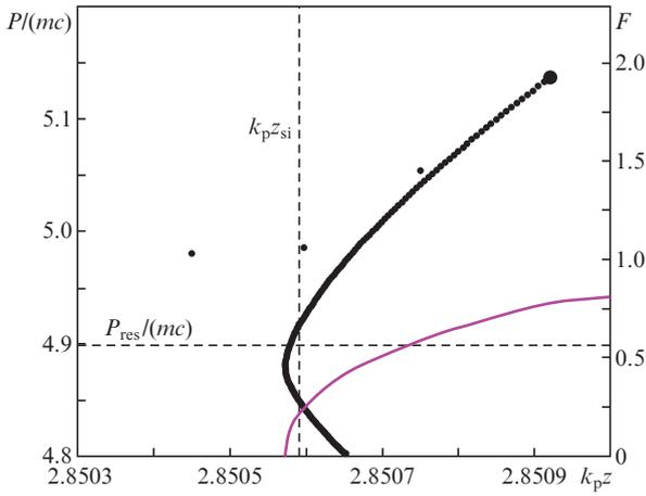
**Figure 2.** Electron distribution on the phase plane  $z, P$  (points) at the instant  $t_b$  of termination of the main self-injection regime. The solid curve is the accelerating force  $F = -|e|E_z/(mc\omega_p)$ , affecting electrons in the wake wave (see the text).
