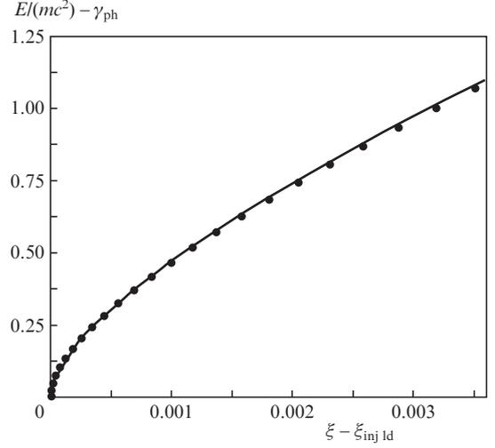
**Figure 6.** Dependence of the energy of the electron-leader accelerated in the wake field on the current value of its phase in the wake wave. Points refer to modelling, and the solid curve is calculation by formula (20).
