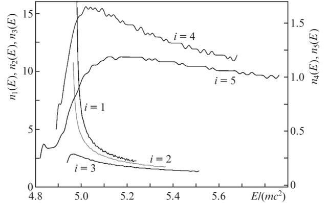
**Figure 4.** Energy spectra  $n_i(E)$  of electrons self-injected into the wake wave at the instants  $t_i = t_b + 0.153\omega_p^{-1}(i-1)$ .
