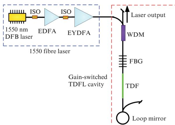
**Figure 1.** Experimental setup of the gain-switched TDFL.
