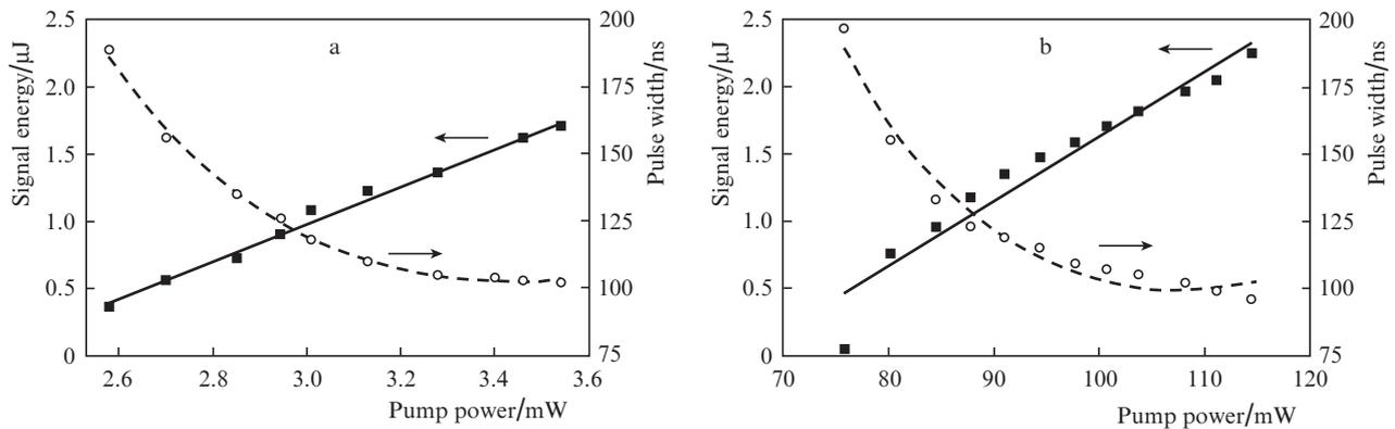
**Figure 4.** Output pulse energy and pulse width vs. pump power in the gain-switched laser at (a) 100 Hz and (b) 1 kHz.
