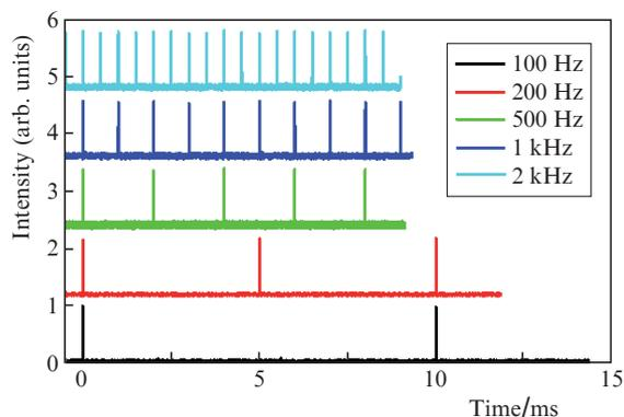
**Figure 6.** Output pulse trains at ultra-low repetition rates.
