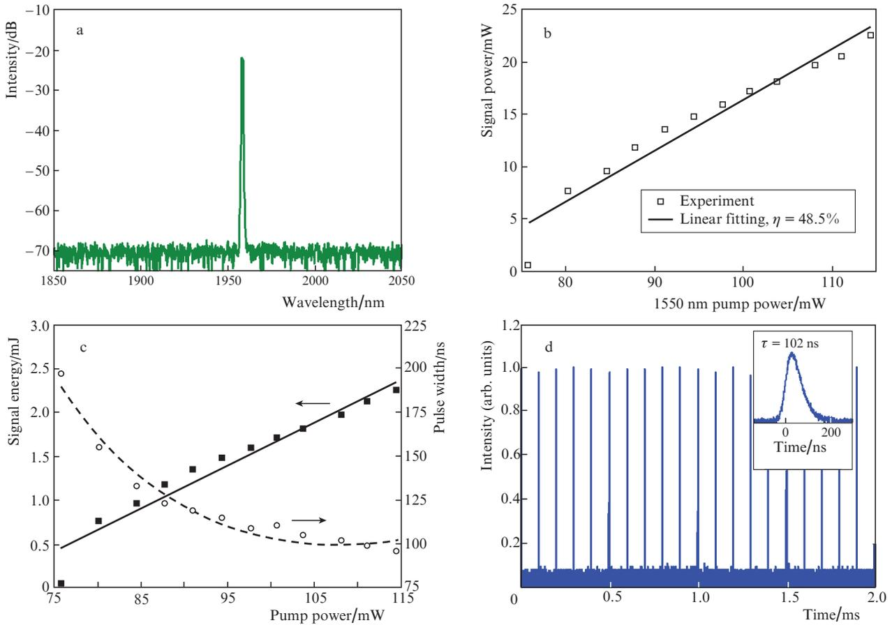
**Figure 3.** (a) Output spectrum of the gain-switched TDFL, (b) output power vs. pump power at  $\lambda = 1550$  nm, (c) output pulse energy and pulse width vs. pump power, and (d) pulse train of the TDFL output at 10 kHz. The inset in Fig. 3d plots the shape of a 102 ns pulse.
