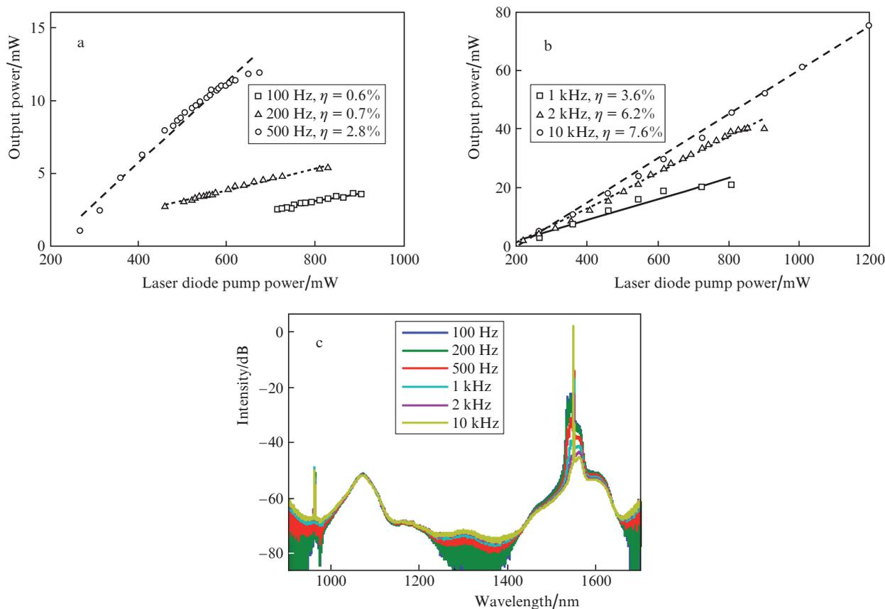
**Figure 2.** (Colour online) (a, b) Power characteristics of the EYDFA at different seed laser repetition rates and slope efficiencies, as well as (c) output spectra at different repetition rates.
