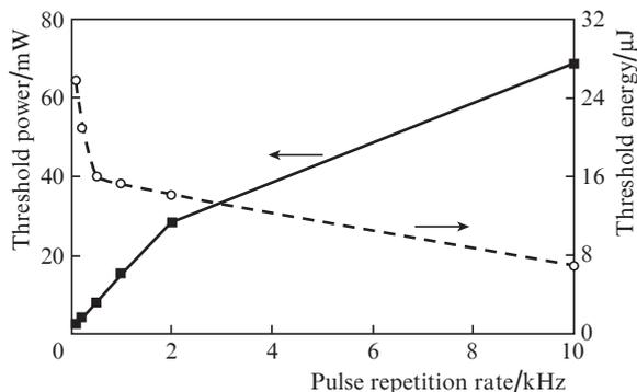
**Figure 5.** Threshold pump power (experiment) and pump pulse energy (calculation) for this gain-switched TDFL at different repetition rates.
