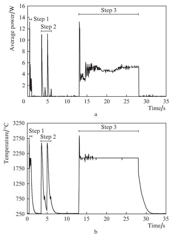
**Figure 4.** Typical oscillograms of (a) the average output laser power and (b) the converter temperature in the process of the formation of an erbium-containing OTFC.
