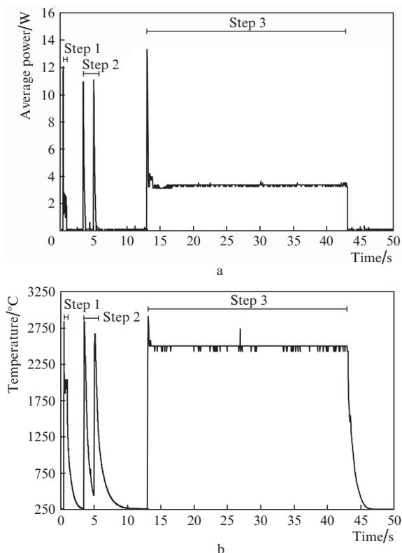
**Figure 2.** Typical oscillograms of (a) the average output laser power and (b) the converter temperature in the process of the formation of a titanium-containing OTFC.
