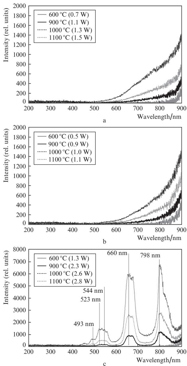
**Figure 7.** Glow spectra of (a) carbon-, (b) titanium- and (c) erbium-containing OTFCs at different temperatures of the converters and incident average powers of a  $980 \pm 10$  nm semiconductor laser.
