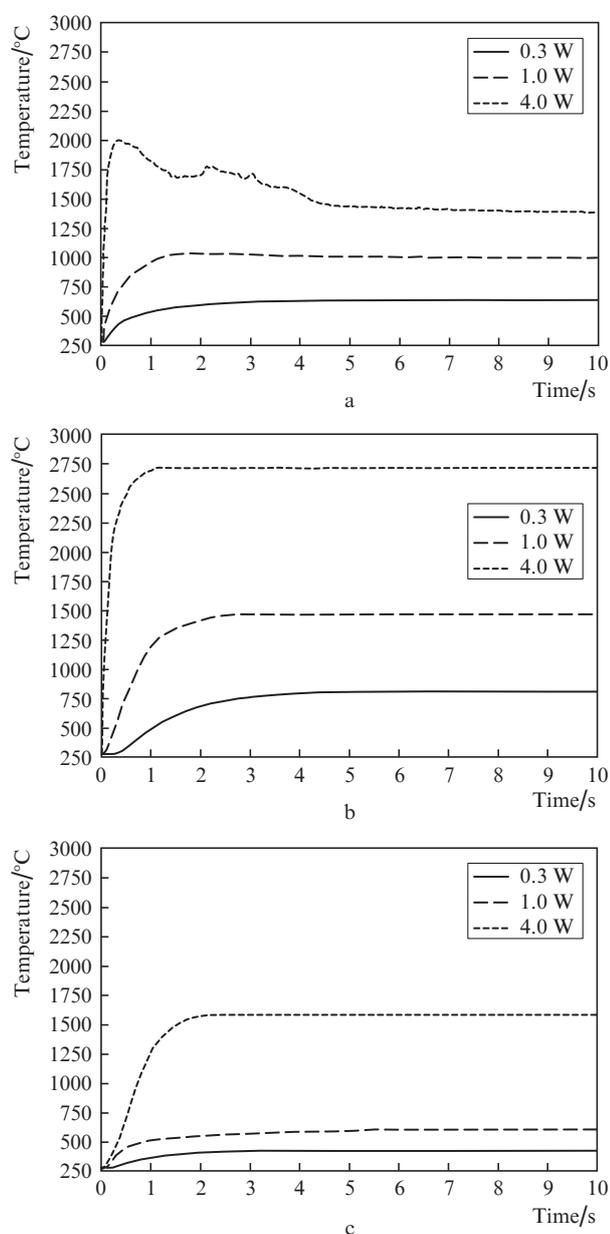
**Figure 6.** Dynamics of laser heating of (a) carbon-, (b) titanium- and (c) erbium-containing converters at different incident average powers of a  $980 \pm 10$  nm semiconductor laser.
