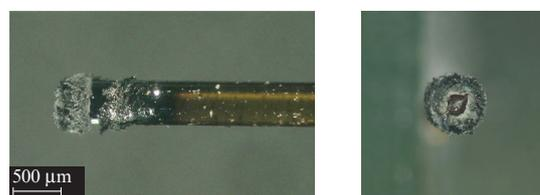
Figure 1. Characteristic appearance of a carbon-containing OTFC.
