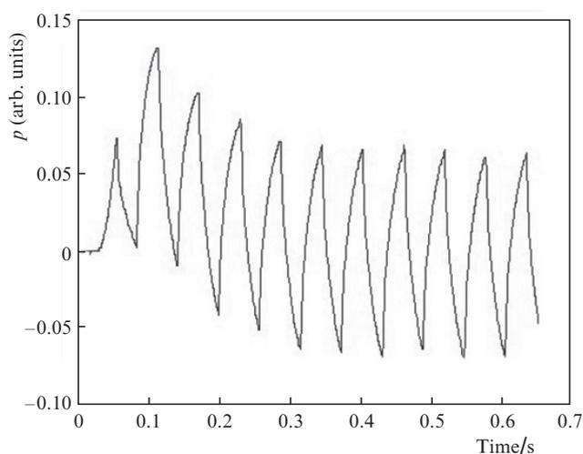
**Figure 3.** Time dependence of the pressure  $p$  in the hydrogel in the process of pulsed laser heating.
