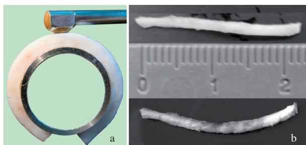
**Figure 5.** (a) Ring-shaped holder of the costal cartilage in the process of its shape modification under the impact of the laser contactor and (b) the costal cartilage of a rabbit before (top) and after (bottom) the laser-induced shape change.
