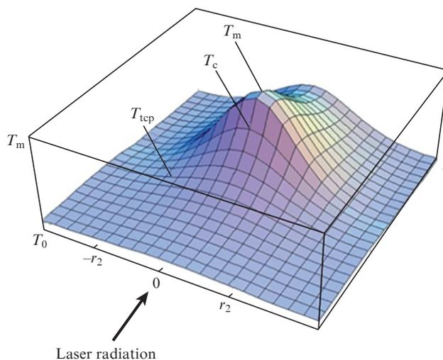
**Figure 2.** Characteristic temperature distribution under laser irradiation of cartilage;  $r_2$  is the radius of the sapphire contactor tip,  $T_0$  is the initial temperature.
