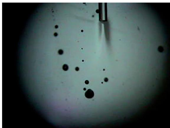
**Figure 4.** Shadowgraph of the laser impact on the tissue-like hydrogel.
