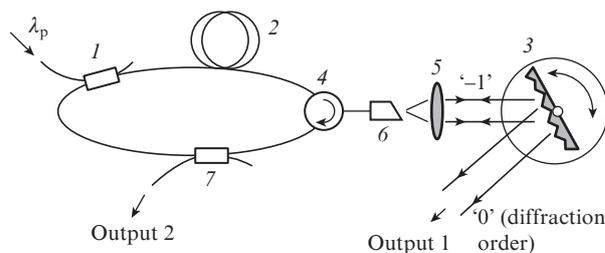
**Figure 1.** Scheme of the tunable bismuth fibre laser: (1) multiplexer; (2) bismuth fibre; (3) diffraction grating on a rotation stage; (4) fibre circulator; (5) microobjective; (6) angle-polished fibre connector (APC); (7) 30/70 fibre coupler.
