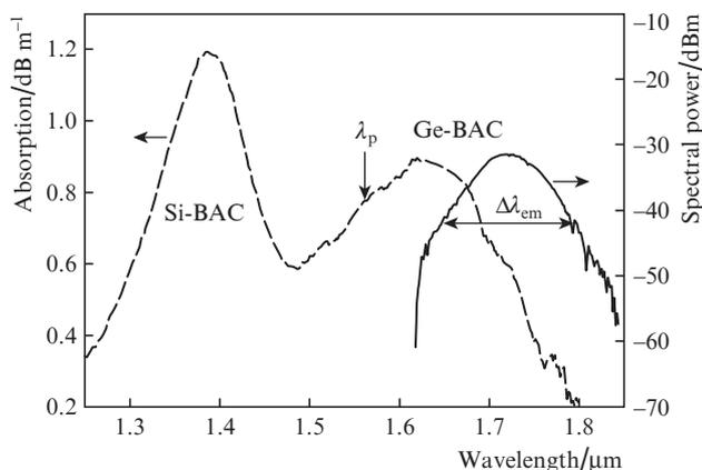
**Figure 2.** Absorption (dashed curve) and luminescence (solid curve) spectra of the bismuth active fibre ( $\lambda_p$  is the pump wavelength,  $\Delta\lambda_{em}$  is the wavelength tuning range).
