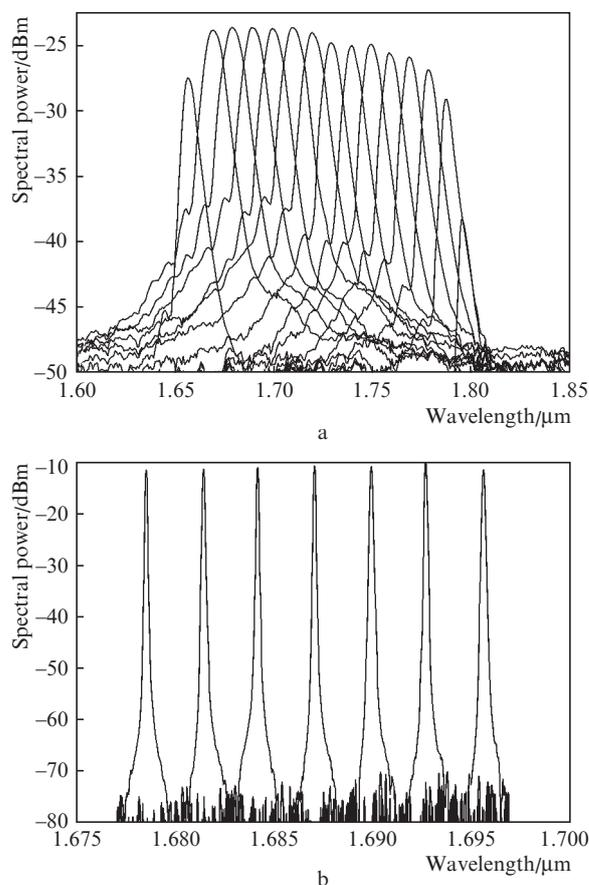
**Figure 3.** Laser spectra measured with a resolution of (a) 10 and (b) 0.02 nm with stepwise rotation of the diffraction grating.
