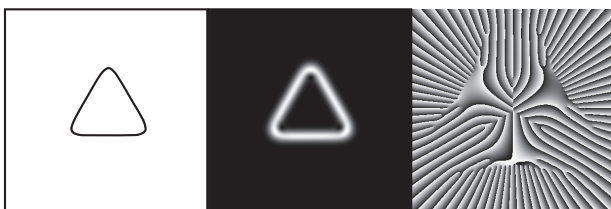
Figure 1. Generating curve and its corresponding distributions of the intensity and phase of the spiral beam.
