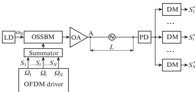
**Figure 1.** Schematic of a fibre-optic OFDM transmission system (see text).
