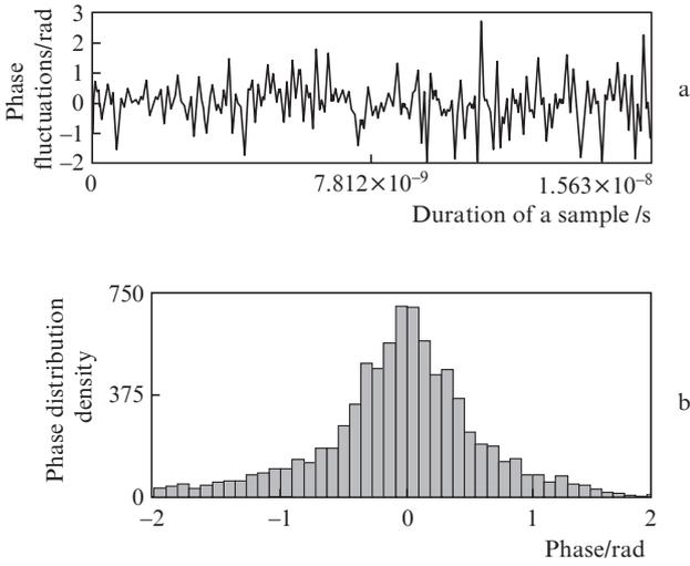
**Figure 3.** (a) Example of phase fluctuations due to XPM during one sample and (b) phase distribution density when  $N = 128$  QPSK-modulated subcarrier channels are transmitted with a frequency spacing of 64 MHz.
