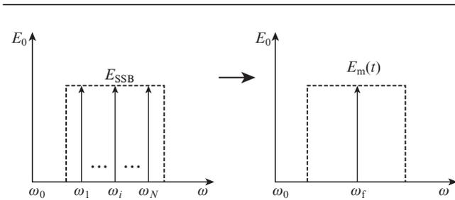
**Figure 2.** Spectrum of the optical OFDM signal.
