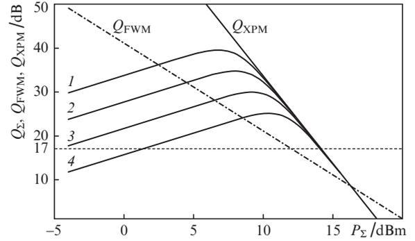
**Figure 5.** Dependences of  $Q$ -factors on the total power  $P_{\Sigma}$  in a 20-km-long SSMF for QPSK-modulated channel subcarriers with a 64-MHz frequency spacing for  $N = (1) 64, (2) 128, (3) 256$  and  $(4) 512$ .
