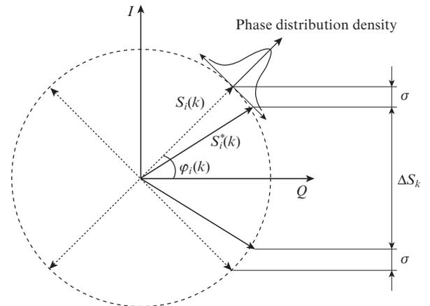
**Figure 4.** Transmitted signal sample  $S_i(k)$  and received signal sample  $S_i^*(k)$ , distorted due to the influence of SPM and XPM, on the  $IQ$  diagram of the QPSK signal.
