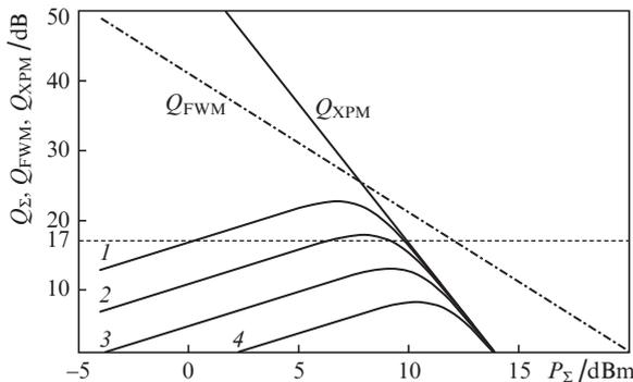
**Figure 6.** Dependences of  $Q$ -factors on the total power  $P_{\Sigma}$  in a 20-km-long SSMF for 64-QAM-modulated channel subcarriers with a 64-MHz frequency spacing for  $N = (1)$  64,  $(2)$  128,  $(3)$  256 and  $(4)$  512.
