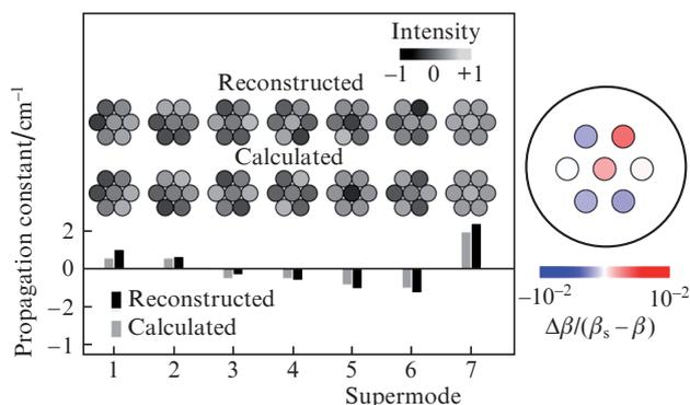
**Figure 3.** (Colour online) (a) Profiles and propagation constants of supermodes and (b) corrections to the propagation constants for each core.
