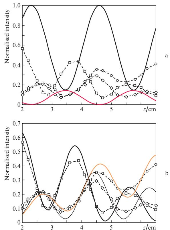
**Figure 2.** Measured (dashed lines) and reconstructed (solid lines) light intensities in cores vs. MCF length for several cores: data obtained using (a) the initial approximation of matrix  $C$  and (b) the best approximation found.
