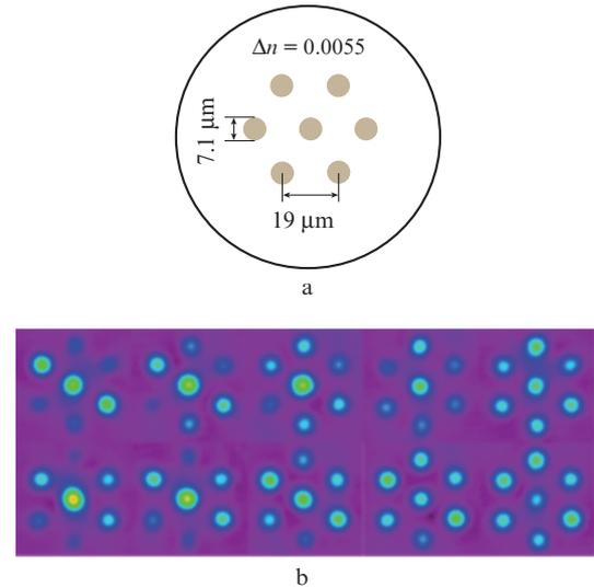
**Figure 1.** (a) Structure of the fibre and (b) examples of intensity distributions visualised using an IR camera;  $\Delta n$  is the core-cladding index difference.
