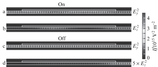
Figure 3. Field distribution in the polarisation rotator in cases (a, b) without voltage at the gold contact and (c, d) with the voltage applied (similarly to the modulator, the latter case is marked ‘off’, which corresponds to a suppressed optical signal). (a, c) Horizontal y -component and (b, d) vertical z -component of the field are shown. Signal in Fig. 3d is amplified by a factor of 5 for better visualisation.
