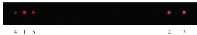
Figure 5. Multiplex hologram responses: 1 is the zero diffraction order; 2, 3 are the 1st diffraction orders; 4, 5 are the responses due to diffraction on the lattice having a difference frequency and resulting from the EC HRM nonlinearity.
