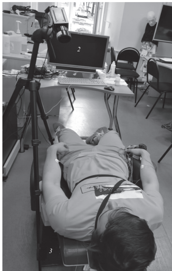
Figure 2. Instrumental diagnostic complex for contactless scanning of the face skin: (1) IR/V-T0831C detector; (2) monitor with a programme of psychoemotional stimuli; (3) chair with backrest tilting drive.
