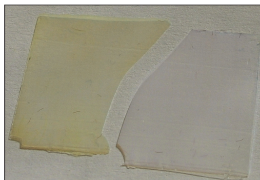
Figure 1. (Colour online) Photograph of photonic crystals P2A-2 with CdSe nanostructures (the left half of the sample, yellow colour) and without them (the right half of the sample).
