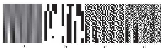
Figure 3. (a) Fragment of the original hologram, the same fragment (b) binarised by the Otsu method and (c, d) represented by random rasters with (c) five and (d) 17 gradations.
