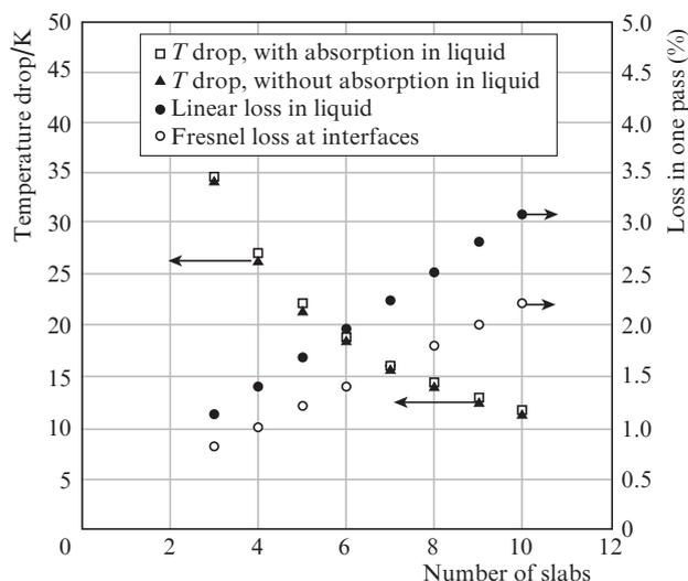
**Figure 6.** Cooling efficiency and radiation loss in relation to the number of slabs. Coolant temperature, 193 K; channel thickness, 0.2 mm; Reynolds number, 44; pressure drop, 106 kPa.
