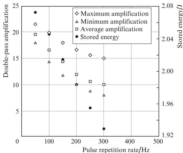
**Figure 11.** Gain and stored energy in relation to the pump pulse repetition rate. The pulse duration is 1 ms, the energy is 4 J.
