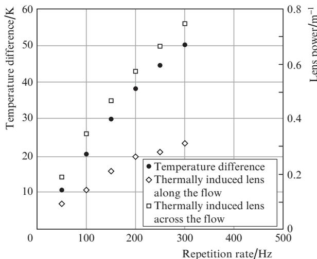
**Figure 12.** Dependences of the temperature difference and the thermal lens power on the pump pulse repetition rate. The pulse duration is 1 ms, the energy is 4 J.
