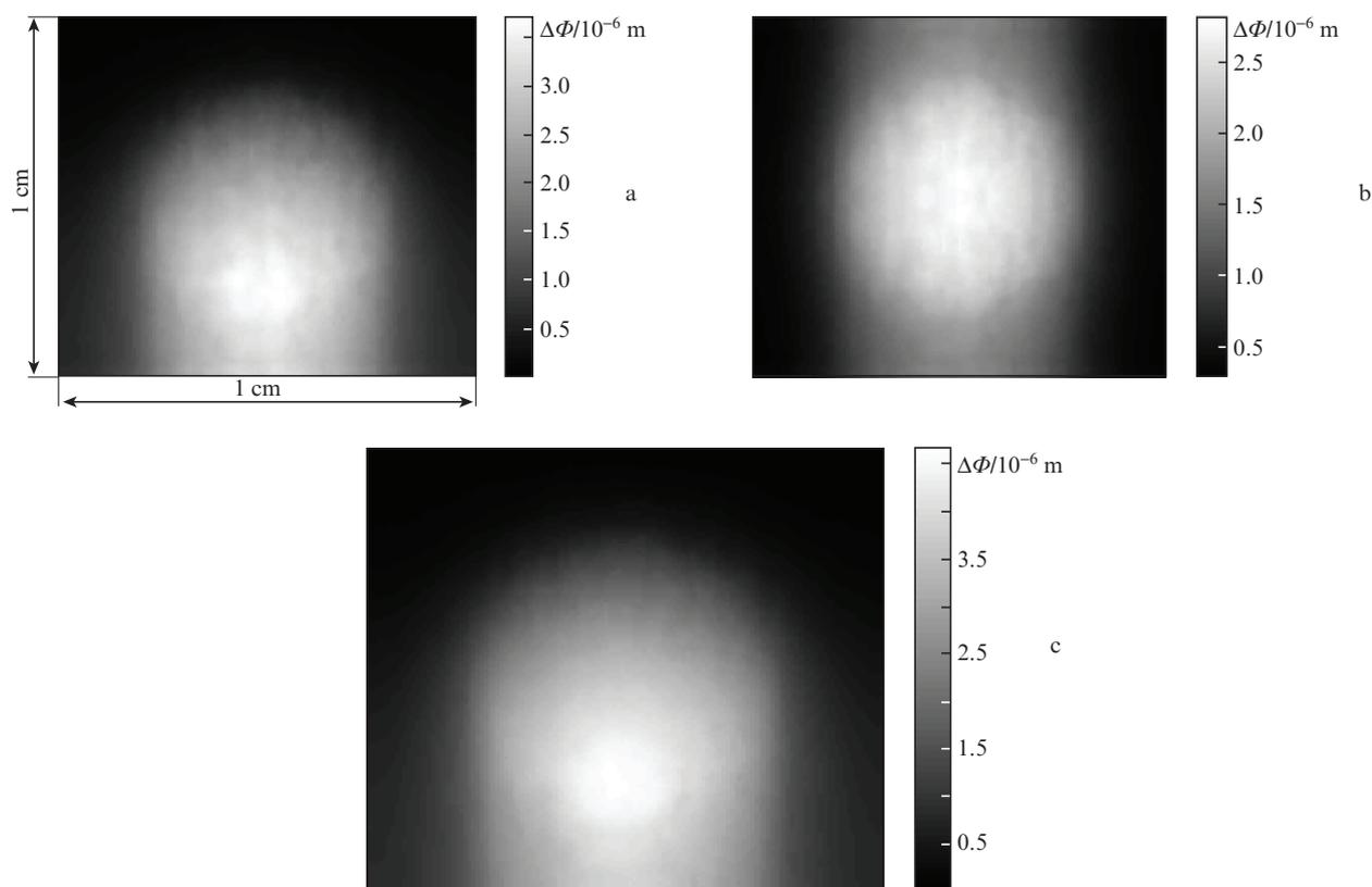
**Figure 7.** Phase distortions in the  $xy$  plane in a laser head in one pass at a coolant temperature of 193 K (a) for a one-way flow and (b) with a counter-flow as well as (c) at 293 K for a one-way flow.
