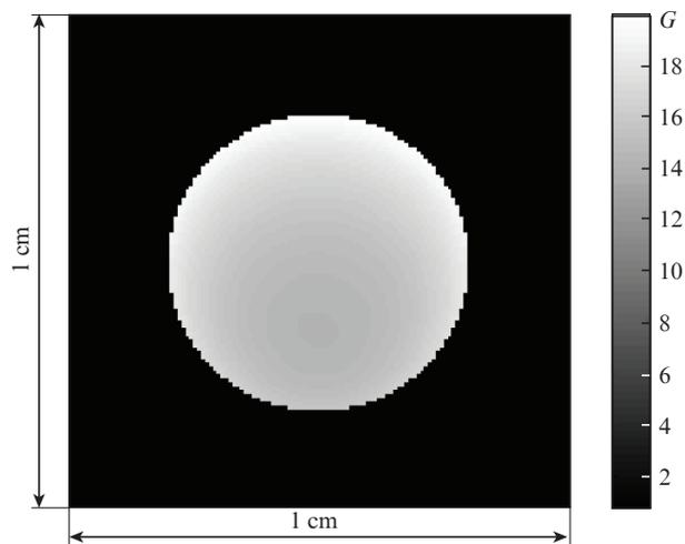
**Figure 9.** Small-signal gain ( $G$ ) distribution in the  $xy$  plane for two passes through the laser head. Peak pump power, 4 kW; pulse duration, 1 ms; repetition rate, 100 Hz; coolant temperature, 193 K; channel thickness, 0.5 mm; Reynolds number, 75.
