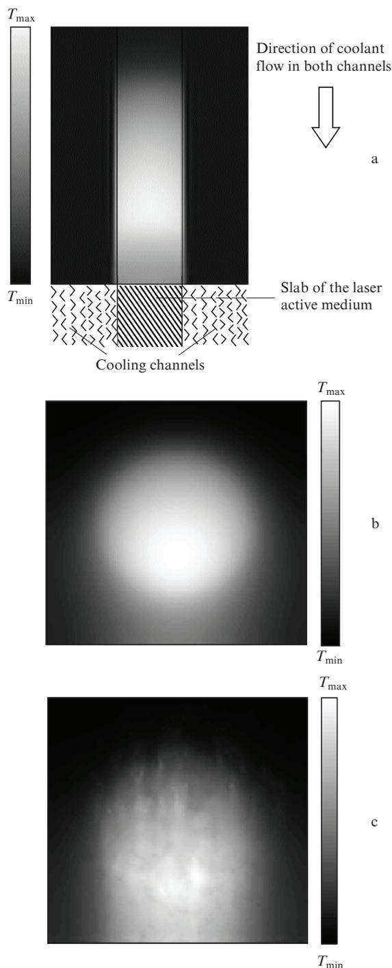
**Figure 5.** Calculated temperature distribution in one slab of the active medium and adjacent cooling channels: (a) two-dimensional section by a plane parallel to the coolant flow and perpendicular to the plane of the slabs; (b, c) two-dimensional section parallel to the slabs (b) in the solid and (c) in the liquid.
