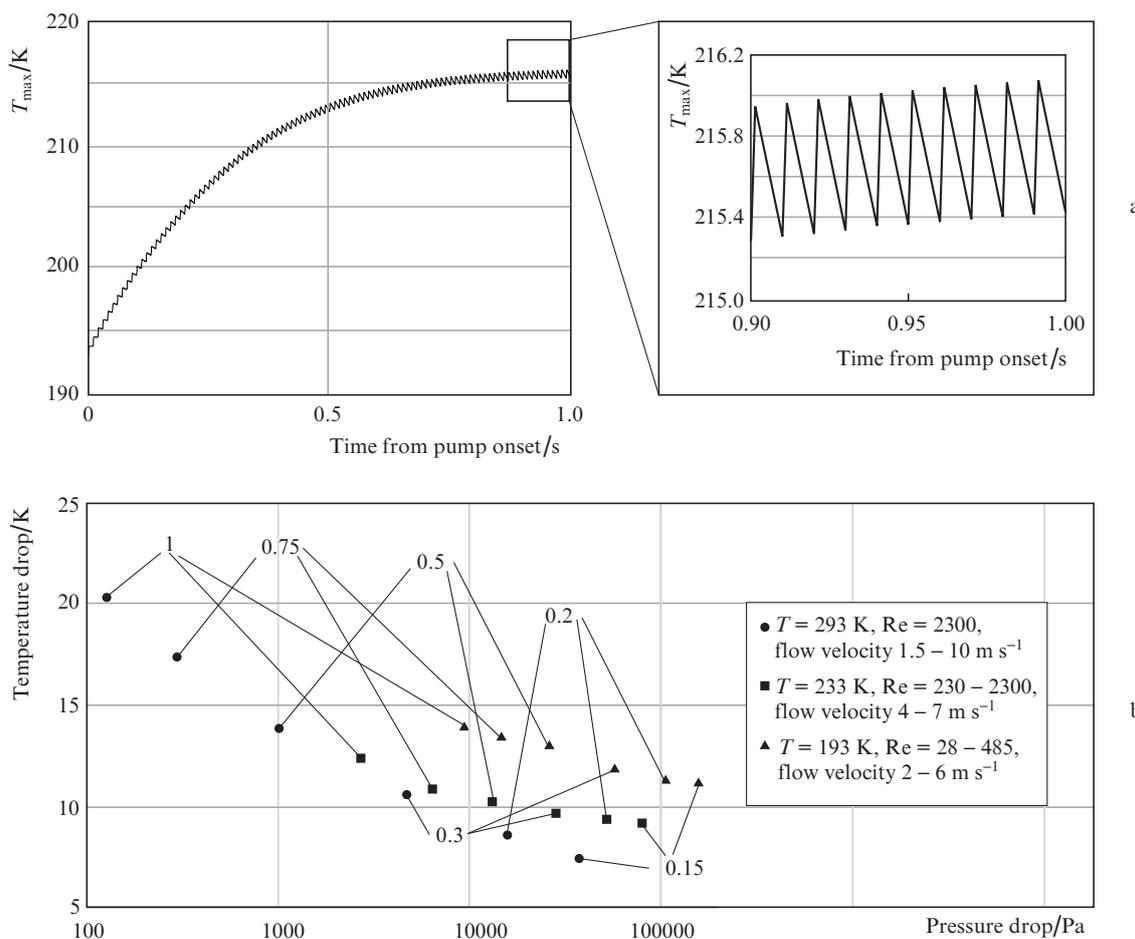
**Figure 4.** Time dependence of the maximum temperature in the active zone (6 slabs 1 mm thick, the channel thickness is 0.5 mm, the pressure drop is 10 kPa); (b) cooling efficiency versus coolant temperature, pressure drop and channel thickness. Channel thickness in millimetres is indicated in the figure.
