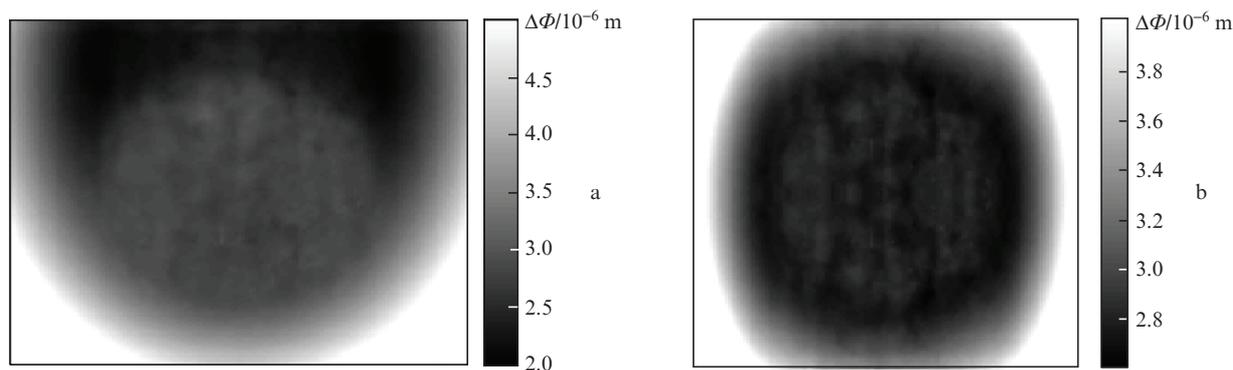
**Figure 8.** Phase distortions in the  $xy$  plane minus the thermal wedge and the parabolic component during cooling (a) with a flow in one direction and (b) with a counterflow.
