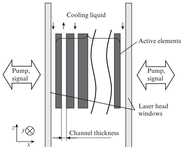
Figure 3. Schematic of a laser head. The light aperture of the laser head is square.
