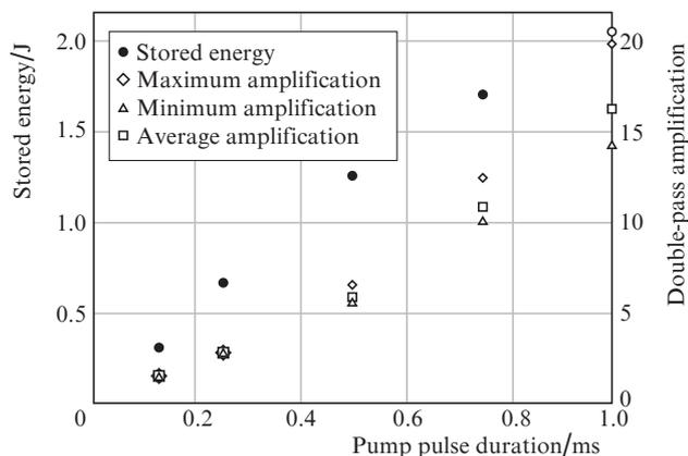
**Figure 10.** Dependences of the extracted energy and the gain in the laser head on the duration of the pump pulse for its constant peak power (4 kW).
