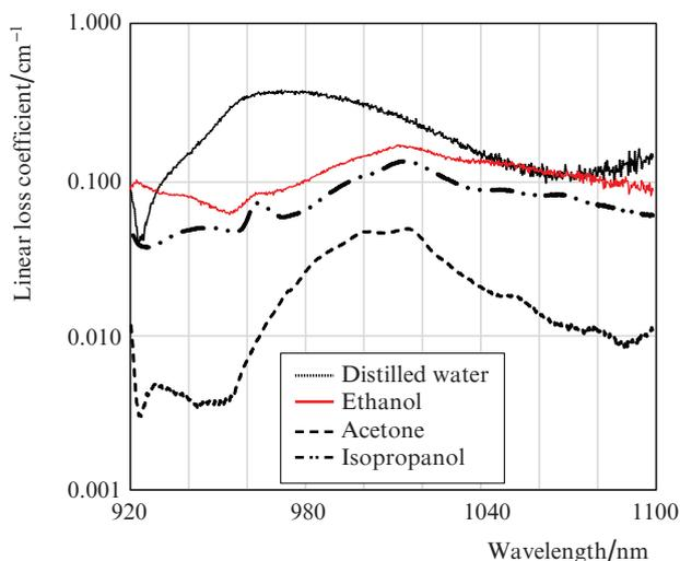
Figure 2. Linear loss spectra in liquids.
