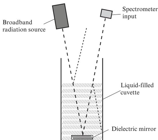
Figure 1. Scheme for measuring the absorption of radiation in a liquid.
