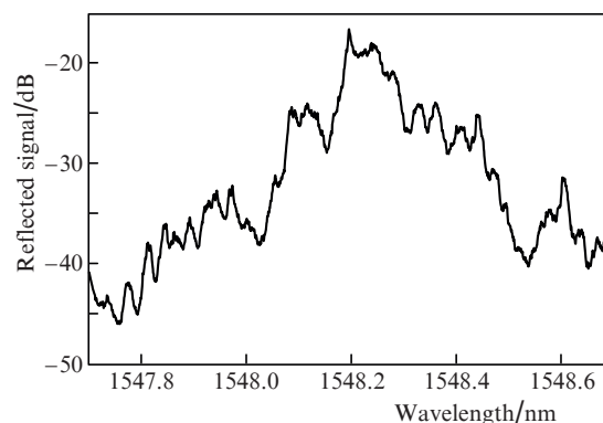
Figure 3. Reflection spectrum of an FBG array inscribed upon drawing a single-mode OF (OF segment length is 1 m).
