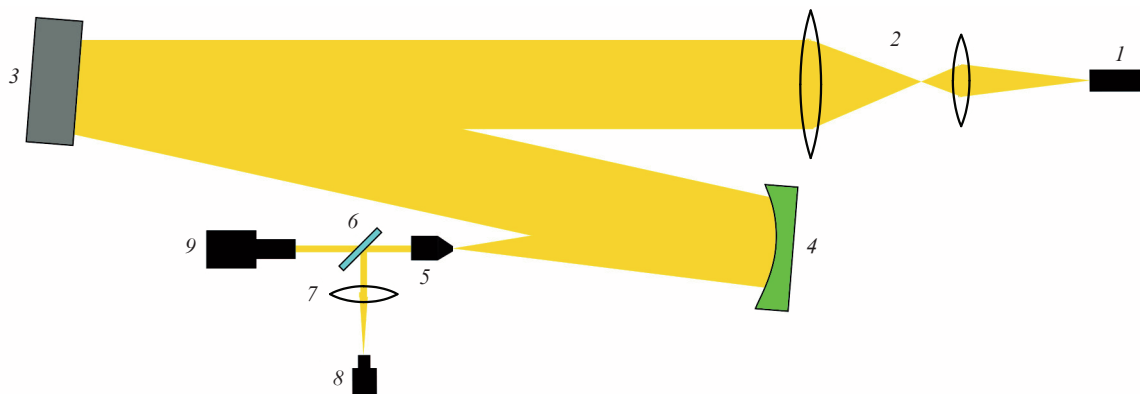
Figure 1. Schematic of the experiment: (1) laser diode; (2) expanding telescope; (3) deformable mirror; (4) F/2.5 off-axis parabolic mirror; (5) microscope objective; (6) beam splitter; (7) lens with a focal length f = 180 mm; (8) far-field camera; (9) WFS.
