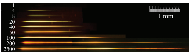
Figure 1. Photographs of luminescent waveguides made of long-lived CCs recorded in LiF under the action of a different number of femtosecond laser pulses with \lambda = 3200 nm. CCs excited by a cw laser with a radiation wavelength of 450 nm make a contribution to the visible luminescence. Femtosecond pulses travel from left to right; numbers on the left are the number of pulses.
