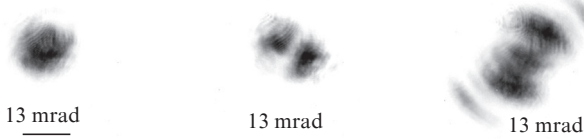
Figure 6. Radiation field patterns in the far-field zone at different laser alignments.
