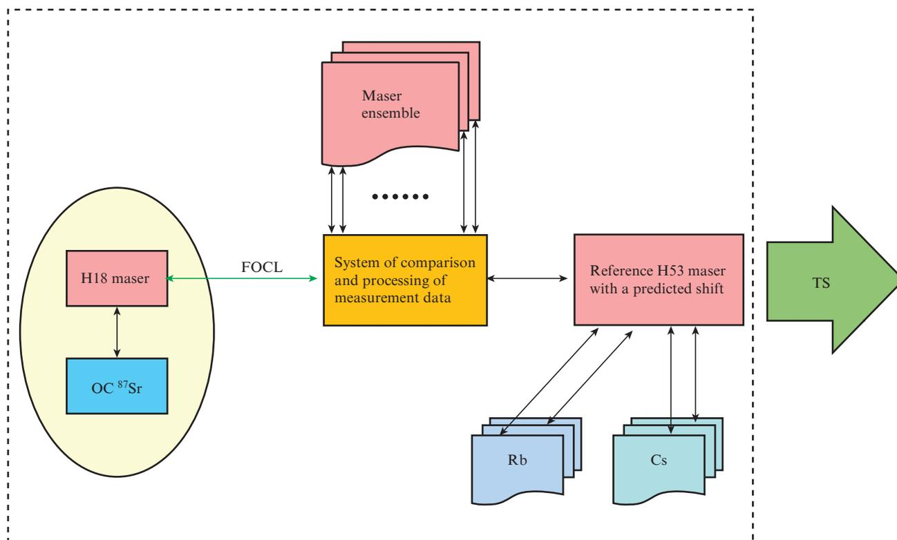
**Figure 1.** (Colour online) General composition of the complex of primary reference frequency standards: (OC) optical clock based on ultracold  $^{87}\text{Sr}$  atoms; (FOCL) fibre-optic communication link; (Cs) primary frequency standard on a caesium fountain; (Rb) frequency keeper on a rubidium fountain; (TS) atomic time scale formed based on comparisons of an ensemble of hydrogen masers with microwave and optical clocks.
