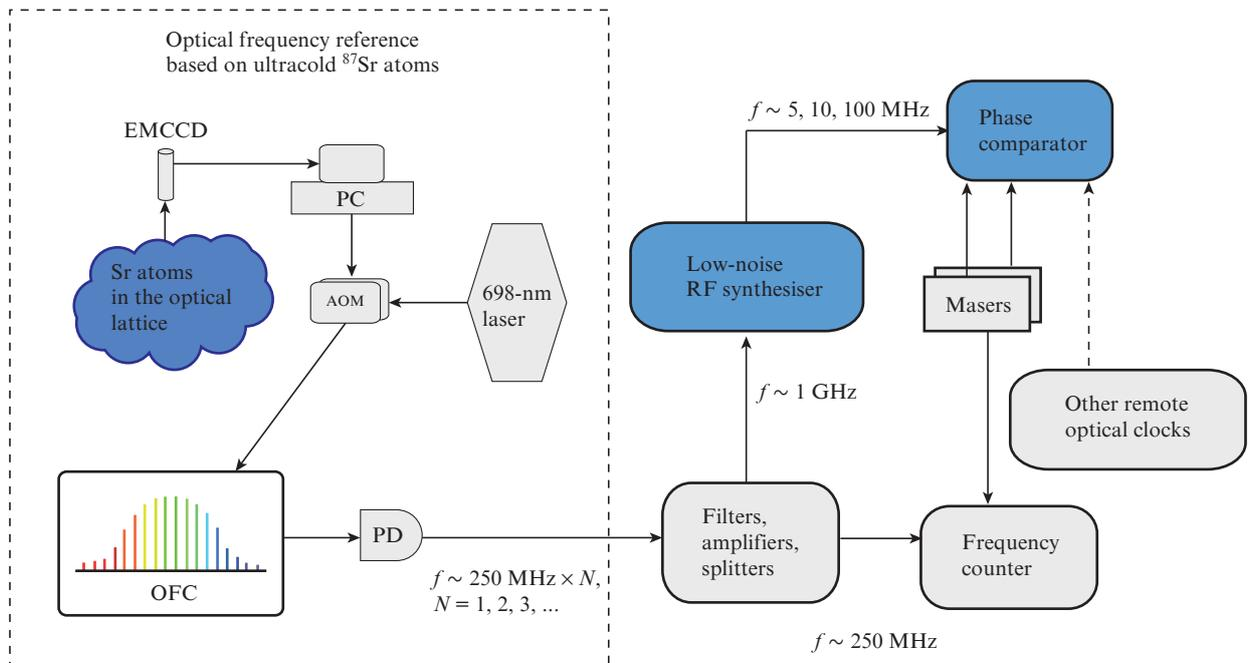
**Figure 4.** (Colour online) Schematic of conversion of an optical clock frequency into the rf range and updated circuit for measuring the converted frequency by a phase comparator:
