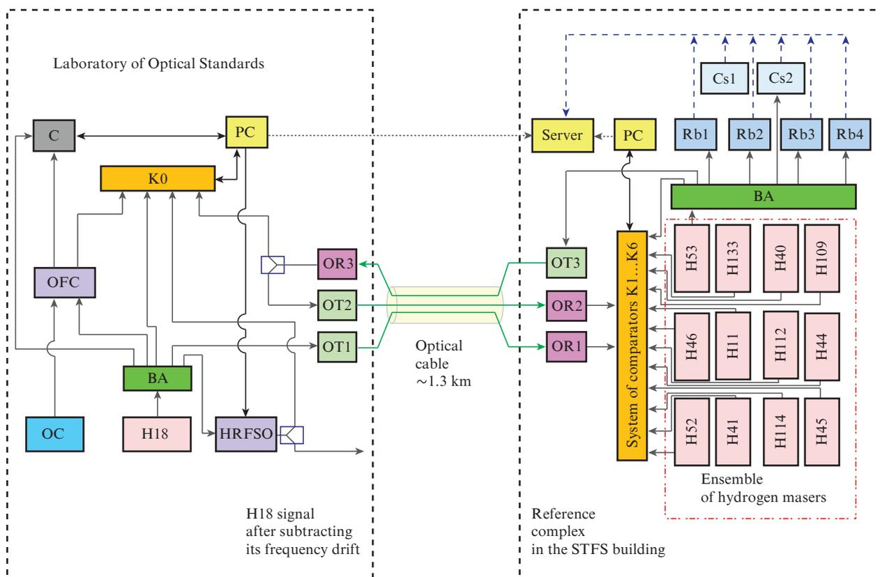
**Figure 3.** (Colour online) Measurement scheme providing comparison with the aid of multichannel comparators of the frequencies of standards entering the main composition of the instrumental complex of the primary standard GET 1-2018:
