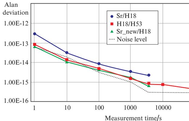
**Figure 6.** (Colour online) Allan deviation of the  $^{87}\text{Sr}$  OC frequency, measured by a frequency counter (circles) and a phase comparator (triangles), comparison of the frequencies of two H masers using a 1.3-km-long fibre-optic link (squares) and the comparator noise level (dotted line). The frequency counter and phase comparator are placed in a constant climate chamber.
