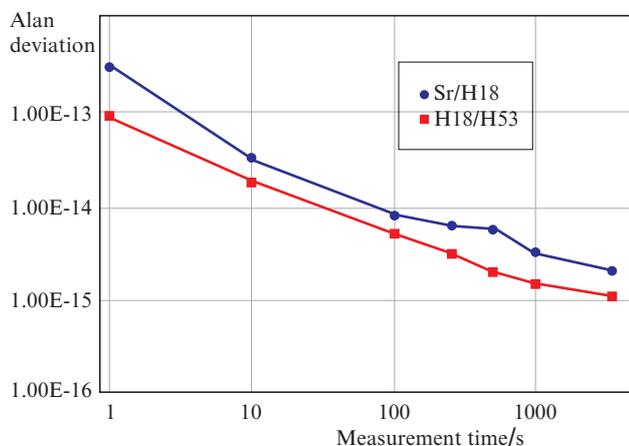
**Figure 5.** (Colour online) Allan deviation of the  $^{87}\text{Sr}$  OC frequency measured by a frequency counter beyond a constant climate chamber (circles) and comparison of the frequencies of two H masers by a phase comparator using a 1.3-km-long fibre-optic link (squares).
